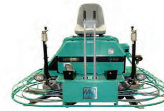
HHNG5 Trowel Rotor Diameter 1168 mm (46 in) Path Width 2335 mm (92 in)
