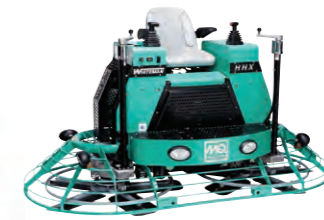
HHXDF5 Trowel Rotor Diameter 1168 mm (46 in) Path Width 2335 mm (92 in)
