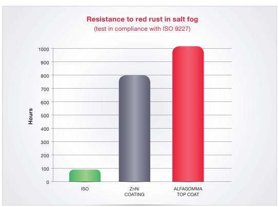
Tested in accordance with ASTM B117-03 and UNI ISO 9227 standards Over 500 hours corrosion prevention in salt spray fog to white rust
